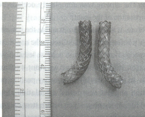
Fig. 2 One of two removed intratracheobronchial stents (Niti-S, nitinol, ID-5 mm, length-4 cm, Taewoong, Korea) is obstructed by granulomatous plug.
